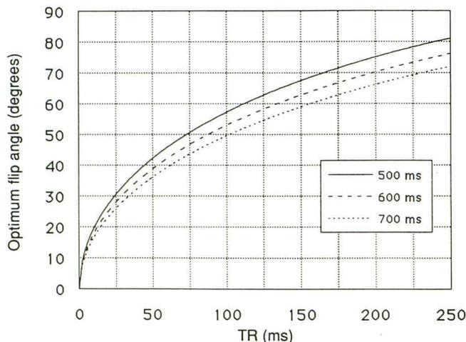
Fig. 1. Optimum flip angle as a function of  $TR$  for the SPGR sequence. Three curves are shown for three different  $T_1$  relaxation times. We felt that these relaxation times are representative of white matter at 1.5 T.
